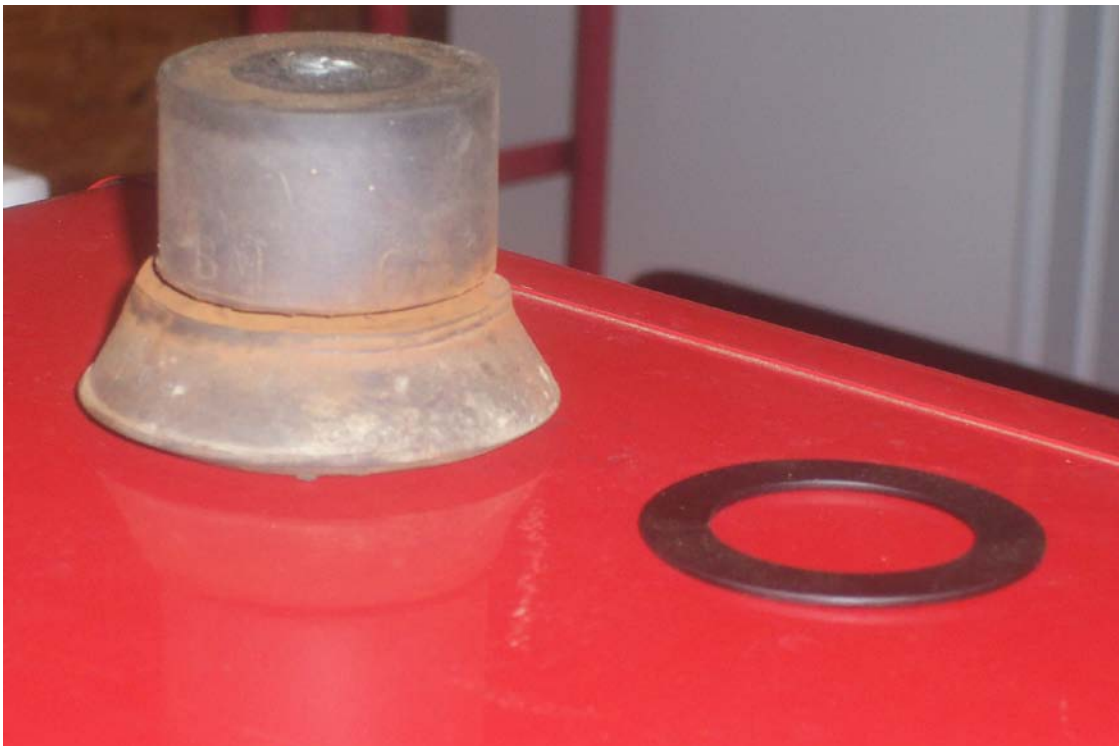
On the left is one of the old mounts. The bottom and top halves of the mount used to be the same diameter! On the right is one of the washers I used to reinforce the body mount areas.
