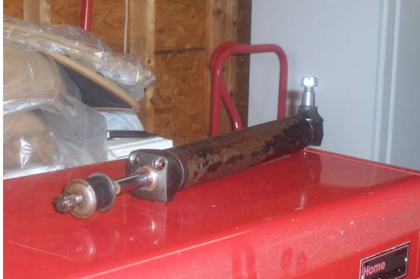
Here is the rebuilt power steering piston.
