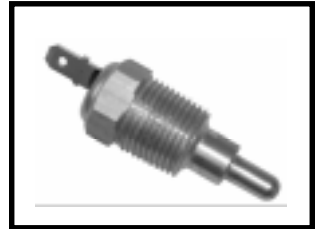
24-0099 ...Engine Temp. Sensor ON 190° - OFF 173° / 1/2" thread
