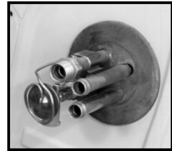
Custom rubber grommet fits in factory blower motor hole for heater and A/C lines.
